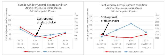
Figure 5: Total Lifecycle Cost (LLC) and energy performance, Central climatic condition, TASK 6
